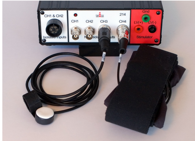
Figure HP-5-S3: The PT-104 and RM-204 connected to an IWX/214.
